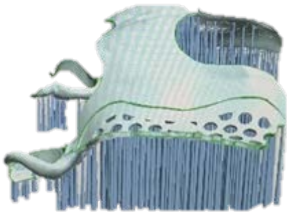
Fig. 8 – Illustration of the supports necessary for successfully laser melting and sintering the removable partial denture framework.
